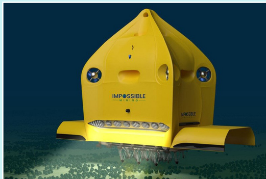
Impossible Metal conducts environmentally responsible harvesting with a hovering robot designed not to dramatically disturb the seabed as it mines. (Source: Impossible Metals)
